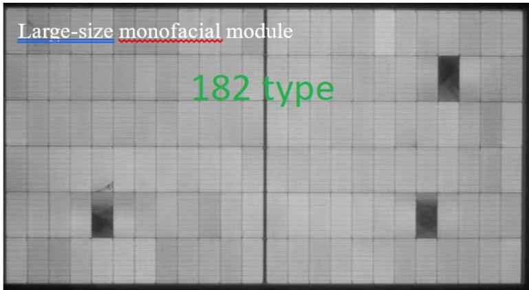
Fig. 2: EL Comparison of large-size (182) and oversized (210) monofacial modules at -2400Pa
